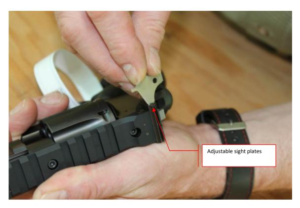
The Super Sport model has two options at the rear sight: Adjustable Sight plates for the light gap and left and right windage screw.
