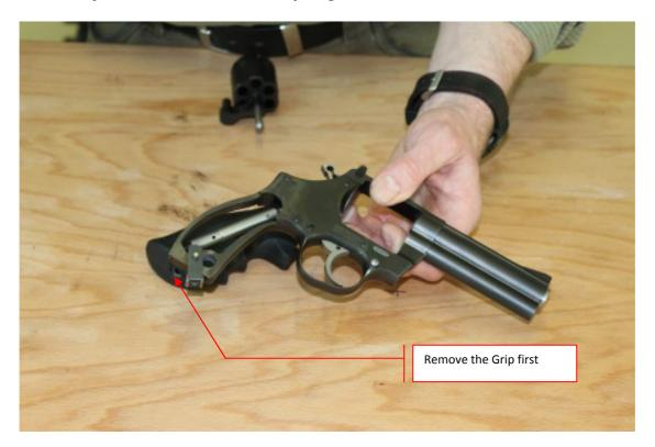
Remove the grip first, after that you can setup the hammermaine spring with an hexagonal tool. Turn it clockwise to make it stronger/ counter clockwise to make it smoother!
