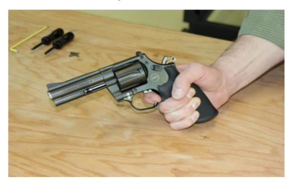
Pulling the trigger cocks the hammer and the shot is fired.
