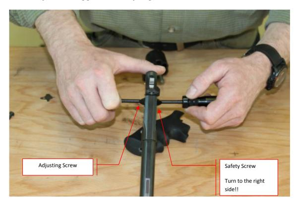
To adjust the trigger rewind spring you have to loose (turn to the right side) the screw on the left side and adjust it with the screw on the right side counter clock wise.
