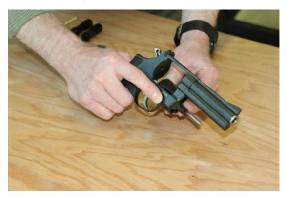
• Remove the cylinder push the button on the right side of the frame.
